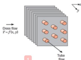
Gambar 2. *Compact Heat Exchanger* [11].
