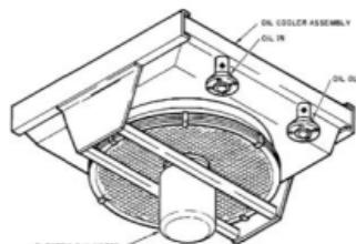
Gambar 1. Tipe *Lube Oil Cooler* [10].
